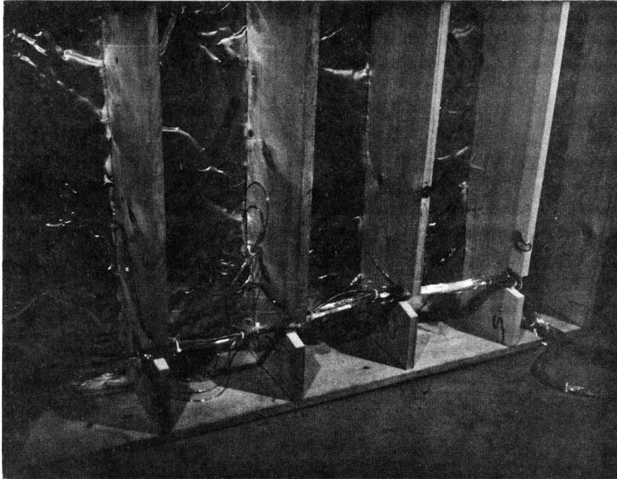
Figure 3-2. Picture of a Portion of Wood Frame Used to Support Aluminum Surface Representing Model Topography.
